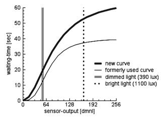
**Fig. 8** Dependency of the duration of the state "wait" on the local illuminance measured by the robot. The bold curve indicates the function used in the experiments described in this article, the thin curve depicts the function used in [26]. The dotted vertical line indicates the median illuminance measured by the robots directly below a bright light; the vertical parallel line indicates the medium illuminance measured by the robots directly below a dimmed light
