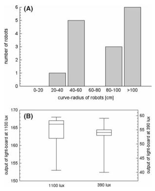
**Fig. 10** (a) Distribution of the robots' side-drifts. Most robots (9 of 15) had no, or only a very slight drift aside with curve-radii greater than 80 cm. Some robots (6 of 15) had a curve radius of less then 60 cm and more than 20 cm. No robot had a curve radius below 20 cm. (b) Median, quartiles and extreme values of measured light intensities (reported sensor values) under constant controlled conditions (1,100 and 390 lux)
