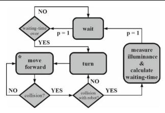
**Fig. 2** State-diagram of our control algorithm BEECLUST. Rounded boxes represent behavioural states of a robot, diamonds identify control structures (if-else) and arrows indicate state transitions. Texts at the arrows indicate probabilities of these transitions (*p*-values) or events that trigger a transition
