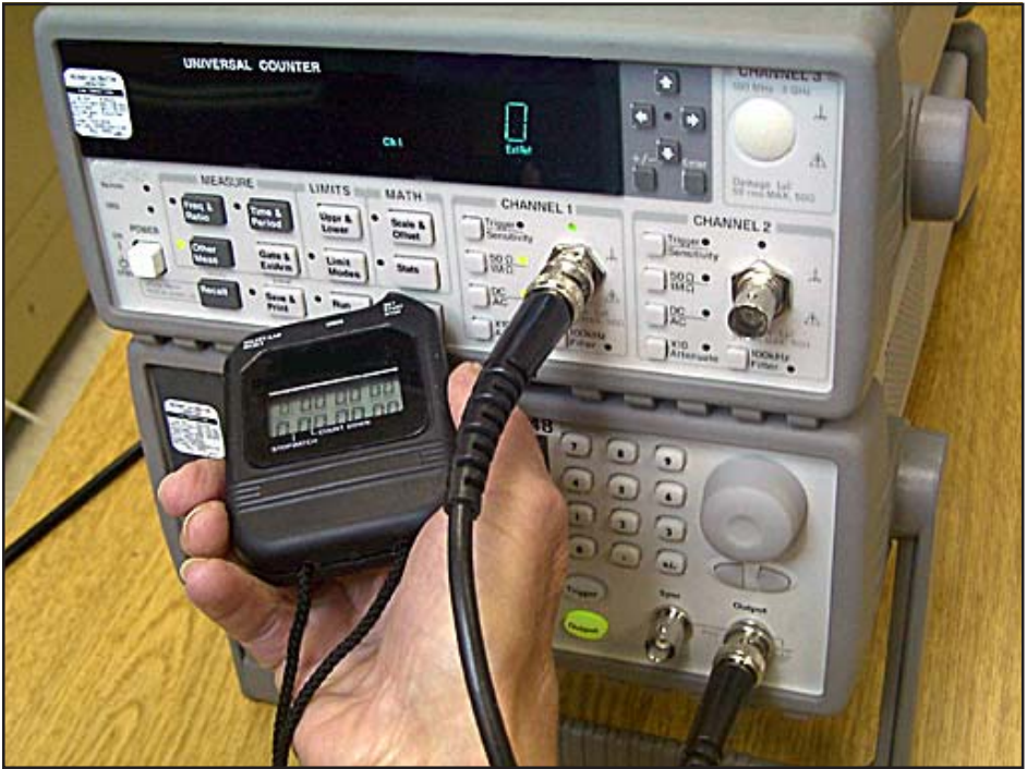
Figure 12. Using the start-stop button of the stopwatch to start the counter.
