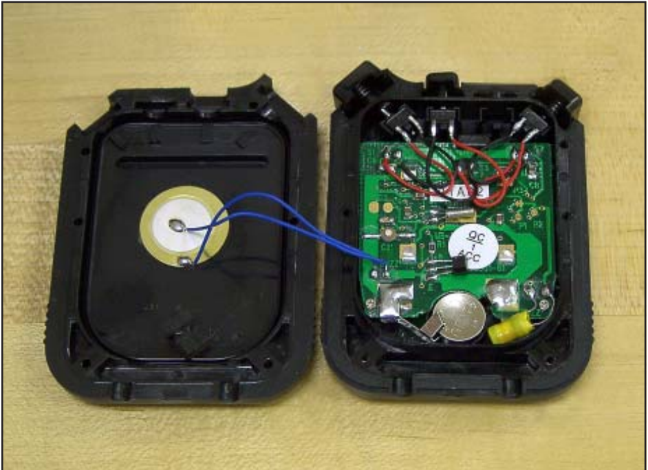
Figure 4. Interior of digital (Type I) stopwatch.
