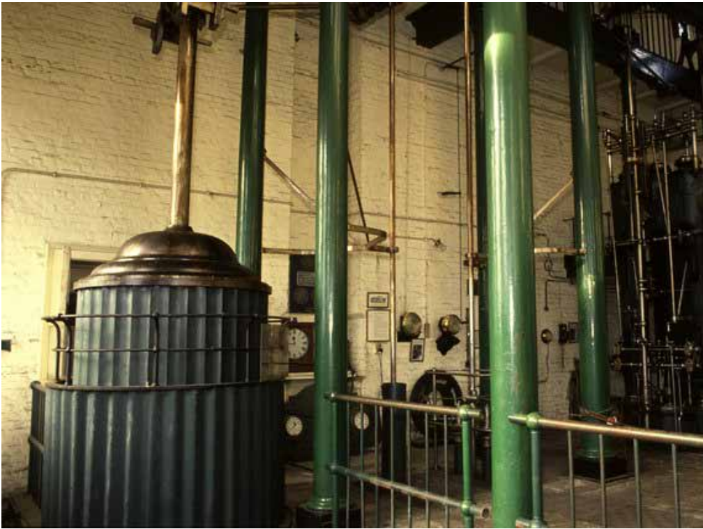
The 1820 Boulton & Watt beam engine, one of two originally installed at Chelsea pumping station beside the River Thames in London and moved upstream to the Kew Bridge pumping station in 1840. (© Chris Allen, Creative Commons)
