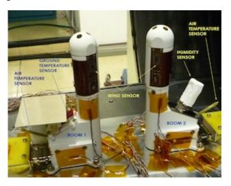
Figure 2: Boom 1 and 2 during the TVT tests. Some calibration tests have been run during TVT. One of them related with the GTS, reason by what a small plate has been place in front of the GTS in order to control the infrared radiation received by it. Regarding the WS, TVT had been used to determine its thermal conductivity losses.
