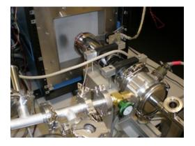
Figure 3: GTS set up for sensor calibration. The main GTS calibration has been carried with the help of a cryostat and a blackbody. Inside the cryostat were reproduced the operational conditions on Mars: low temperature, low pressure and carbon dioxide atmosphere. The black body placed in front of the sensor was the infrared radiation reference.
