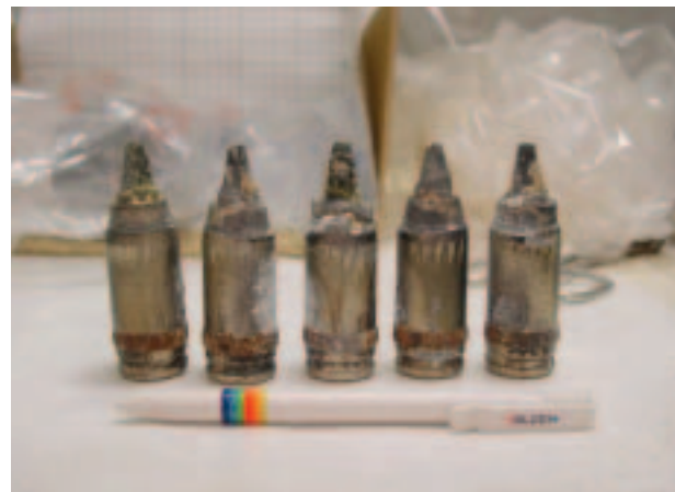
FIG. 2. Penetrators collected by the RPD and analysed at the Agency's Laboratories at Seibersdorf.
