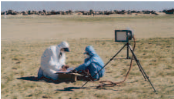
FIG. 12. Air sampler with filter holder and filter.
