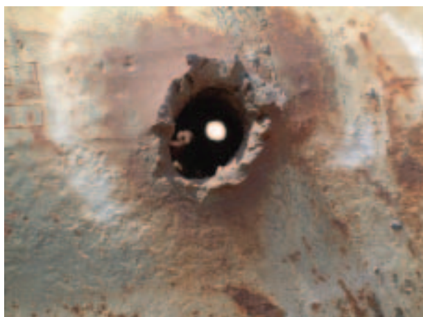
FIG. 7. Hole caused by the impact of a DU munition in a tank stored at Um Al Kwaty.
