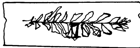
Figure 1.41: Piping in weld.
