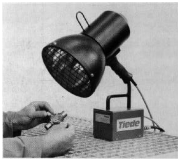
Figure 4.18: Portable 100 W mercury arc black light source.
