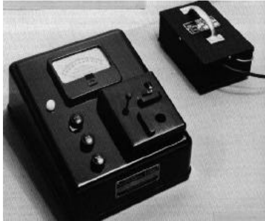
Figure 4.22: Laboratory-type fluorometer specified by MIL-I-25135 containing built-in black light source and interchangeable for light modification.
