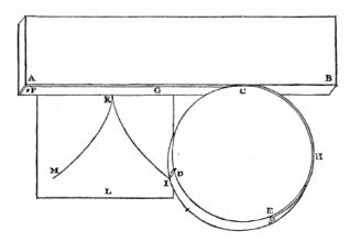
pendulum; and F G H E is a small bandage, or better a thin metal foil, fixed to the rule at the point F of this, and to some point of the circumference of the cylinder E, thus in order that it shall be partially wrapped around the cylinder alongside the rule A B. Moreover a sharp iron point DI shall be fixed to the cylinder, projecting a little below the base, and thus in order that the circumference of the cylinder corresponds exactly to it. [p. 11]
