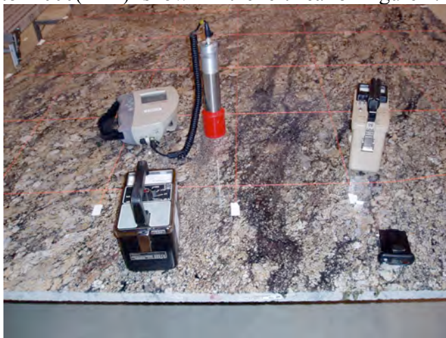
Fig 1 Scintillation-based gamma detectors used for pre-screening
