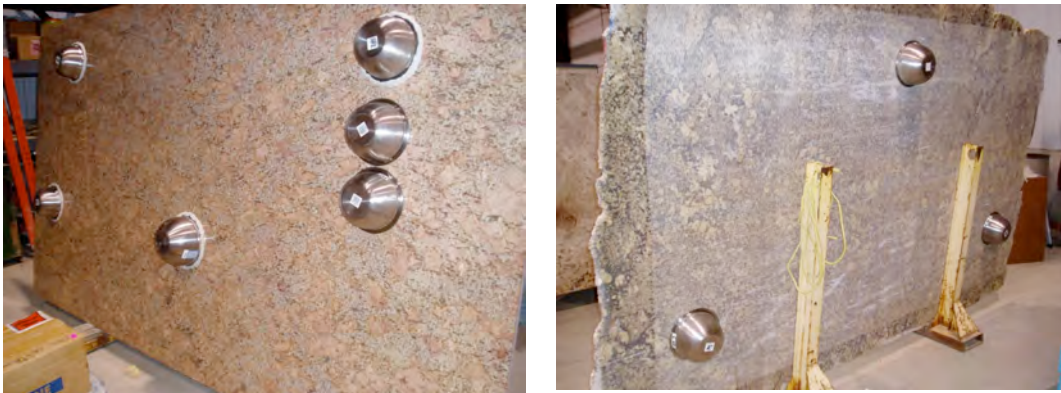
Fig 3: Emanation measurements on slabs. The slab on the left is an example of a netting glued to the non-polished side.
