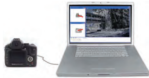
Fig. 3. In our prototype implementation, a laptop is connected to a camera. The laptop computes the relative camera pose and visualizes how to translate the camera with two 2D arrows. Our alignment visualization, which consists of edges detected from the reference image composited onto the current view, helps users to evaluate whether they have reached the final viewpoint.
