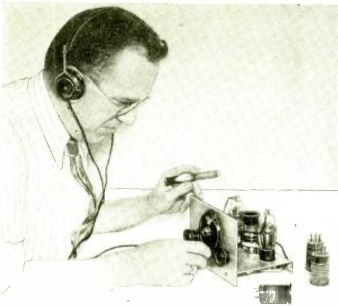
Front view of the 2-tube "Pentaflex," which uses two 2A7 or 6A7 tubes.
