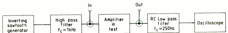
Fig. 4. Block diagram of measurement setup
