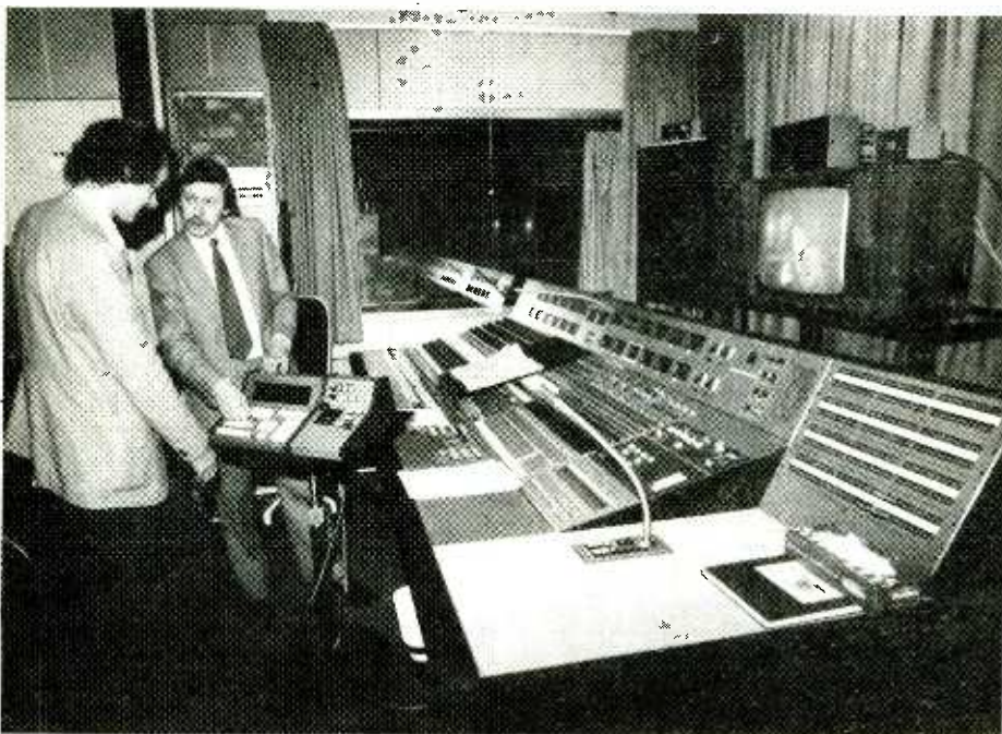
Terry Newbery, of the BBC Studio Capital Projects Department, discusses the Sypher-2 sound-synchronisation system with Mike Jones, a sound supervisor. On the right is computer-assisted mixing console made by Neve which includes the control units for the Sypher-2 system.
