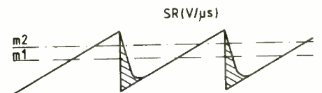
Fig. 2. Input sawtooth and response of amplifier
