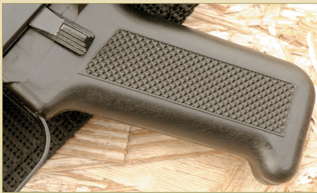
The SA M-7 SF side-folder uses a selector much like the Galil ARM's. A vertical lever on the left side of the pistol grip can be manipulated to operate the selector.
