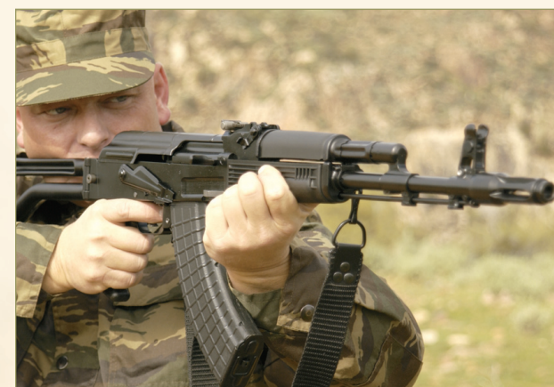
The SA M-7 SF has a side-folding stock and represents the AK configuration currently in service with the Bulgarian armed forces. It's as rigid as a fixed stock.
