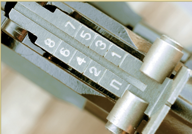
The sliding tangent rear sight is adjustable for elevation to 800 meters in 100-meter increments. The battle sight setting (the Cyrillic "P") is equivalent to 300 meters.
