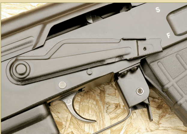
The selector lever and a flapper-type magazine catch/release are standard AK features. Kokalis counts the selector one of the AK's weak points, as it is noisy.
