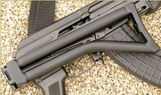
When folded to the right, the SA M-7 SF buttstock is securely retained by a spring-loaded catch/release on the receiver. This is a study, rugged folding stock.
