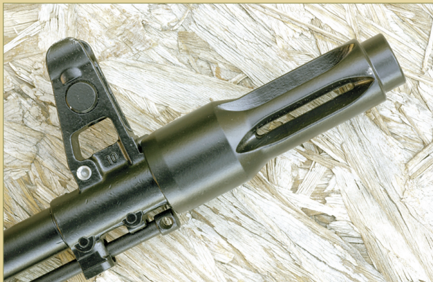
The SA M-7 side-folder and SAS M-7 A1 down-folder both have a removable flash hider, 80 mm in length, with four longitudinal slots. The Classic has a muzzle nut.
