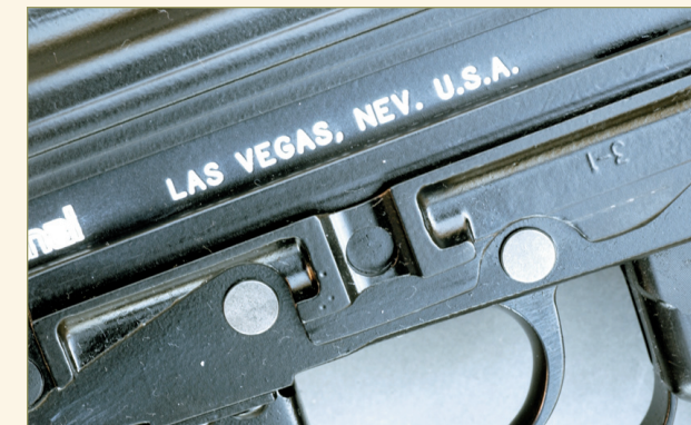
The SA M-7 SF side-folder is equipped with the conventional Soviet-type side rail for mounting optical devices. Kokalis recommends the Kobra red dot sight here.
