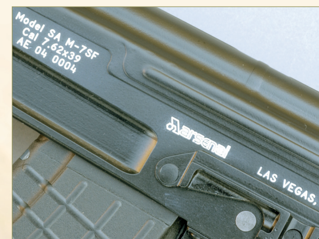
Markings found on the SA M-7 SF drop forged receiver: Kokalis says that the forged receiver is ideal for the sporting user, as it is stiffer than the stamped.
