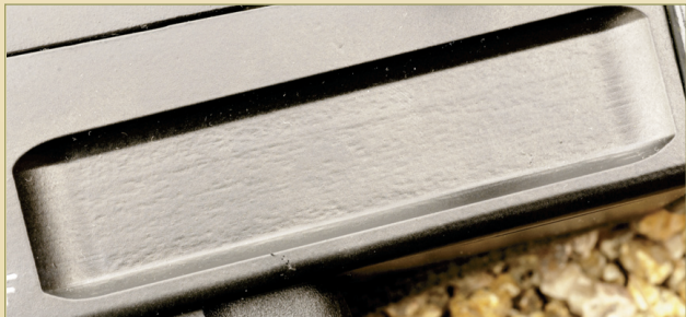
Forged receiver AK47s all have a distinctive rectangular lightning mill cut directly above and forward of the magazine well on both sides of the gun's receiver.
