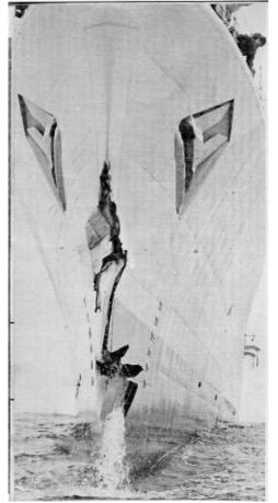
Frigate v Gunboat. The Naiad's damaged bows (above) and the cause (below), Tyr trying to cross her bows to cut the trawl of "Irvania".
