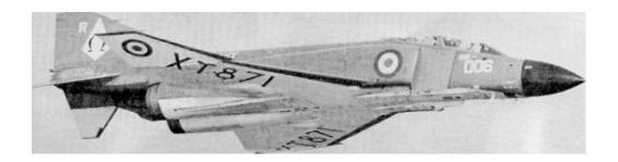
**PHANTOM** (above): The fabulous Phantom, operated by 892 Squadron, is an all-weather fighter aircraft developed in America and adapted for use in the Royal Navy. Two Rolls-Royce Spey engines with after burner allow speeds over Mach 2 and its predecessors hold no less than 15 world records for speed and rate of climb. The aircraft you can see comes from the Fleet in Reserve pool based at RAF Leuchars. Scotland.
