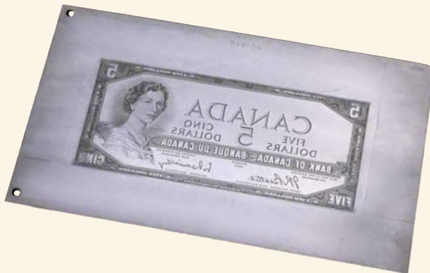
Master plate for the 1954 $5 note. This was used to prepare the full printing plate of 32 notes
