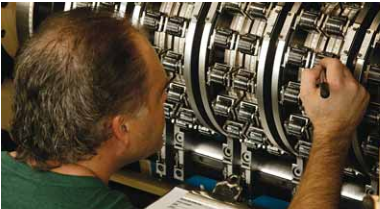
A numbering apparatus mounted on the printer automatically advances one number with each printing cycle, giving each bank note a unique serial number.
