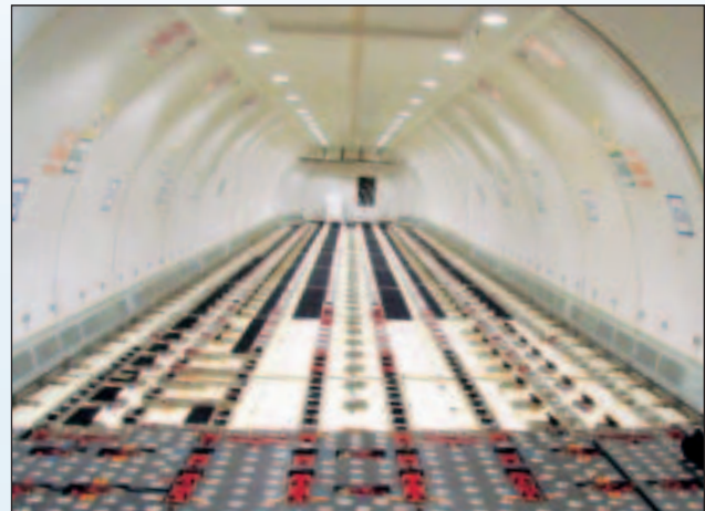
Main Deck of the B767-200ER
