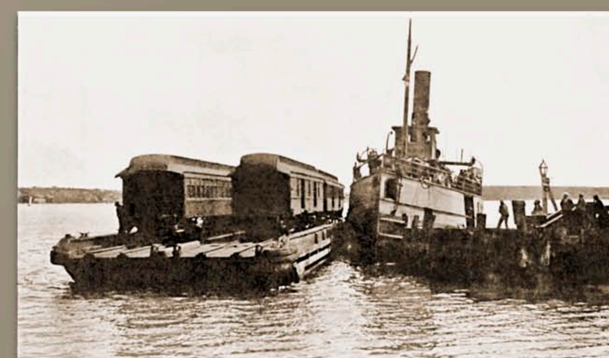
The S.S. Mulgrave, a towboat, was used to transport railcars by barge from Mulgrave to Point Tupper from 1893 to 1902 until the S.S. Scotia rail ferry service began.
