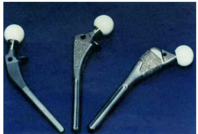
Fig. 5. Medical-grade alumina used as femoral balls in total hip replacement. Note three alternative types of metallic stems used for morphological fixation. (Photograph courtesy of J. Parr.)
