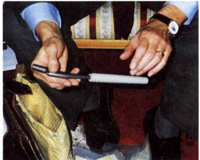
Fig. 20. PE-HA composite used as a sleeve for the stem of a total hip implant. (Photograph courtesy of W. Bonfield.)
