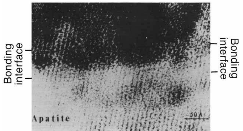
Fig. 17. TEM micrograph using lattice imaging to show epitaxial bonding between (bottom) HA implants and (top) the HA phase of bone. (Photograph courtesy of M. Ogiso.)
