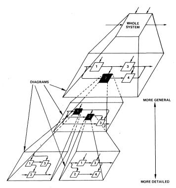
Fig. 1. Structured decomposition.
