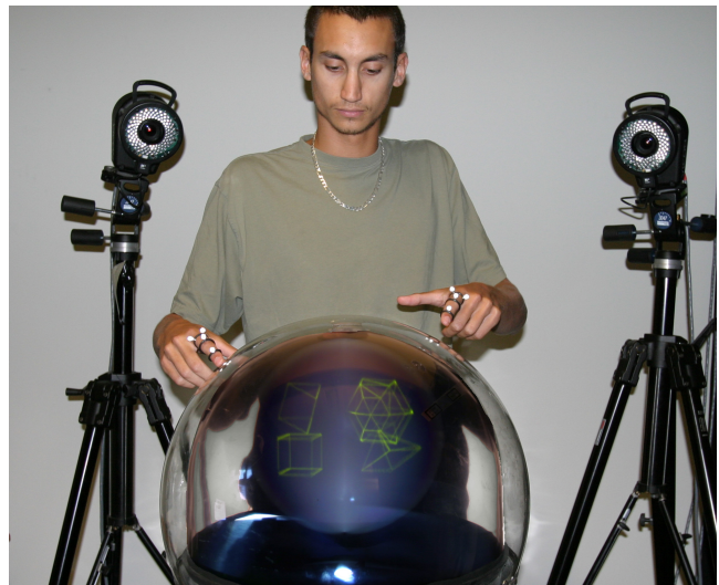
Figure 1. User working with a volumetric display, with finger input tracked using a camera-based motion tracking system.
