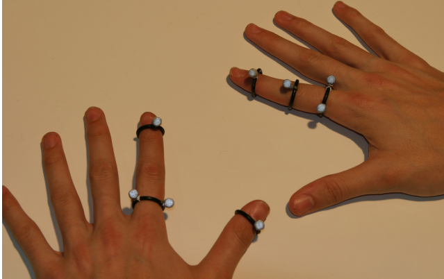
Figure 3. Markers used for tracking finger positions. Multiple markers enable us to track bending of the index fingers, as well as finger tip position and orientation.
