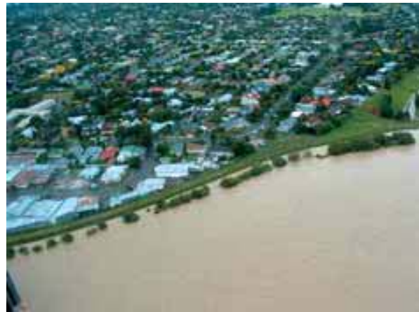
The $7 million Fitzroy Bend protection stopbank in Palmerston North proved to be money well spent on reduction. The town's investment neutralized a potentially devastating flood.
