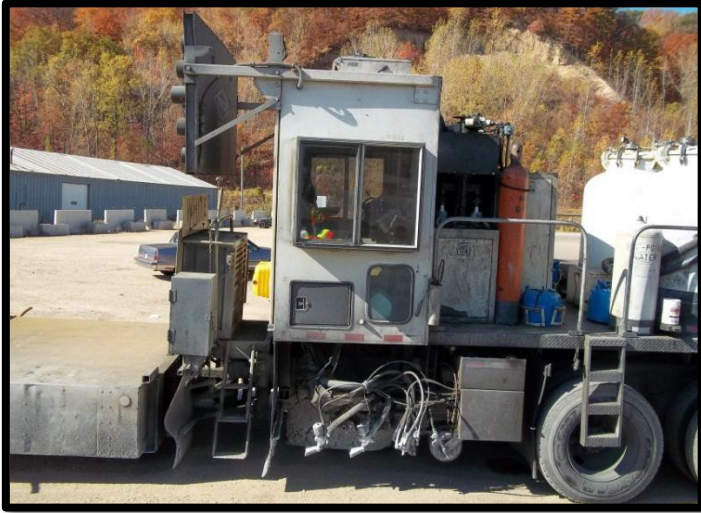
Figure P-3: Pavement Markings Truck - Striper Cab
