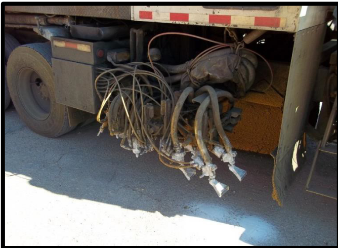
Figure P-4: Pavement Markings Application Carriage
