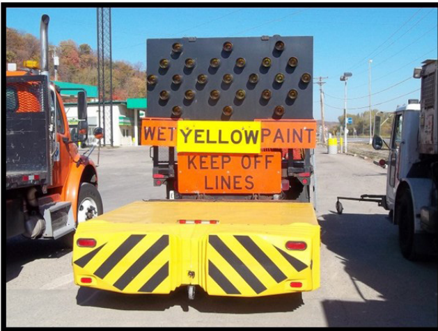
Figure P-6: Attenuator Truck with Arrow Board
