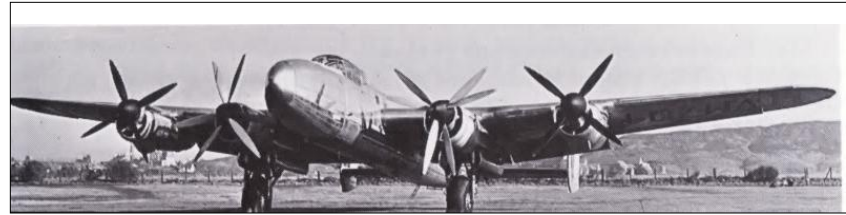
Lancastrian VM704 with Griffon C-props inboard, Merlin 100 series engines for Avro Tudor outboard
