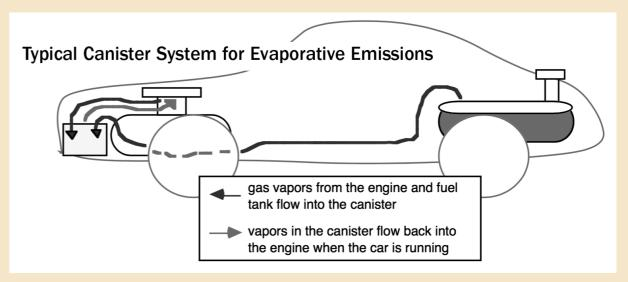
**Controlling evaporative emissions.** These controls prevent evaporation of gasoline (VOC), reducing pollution with a net cost savings.
