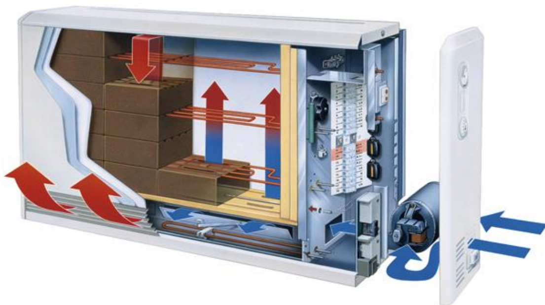
Figure 20 - Structure of a dynamic storage heater - Source: http://www.storageheaters.com/how-storage-heaters-work.htm
