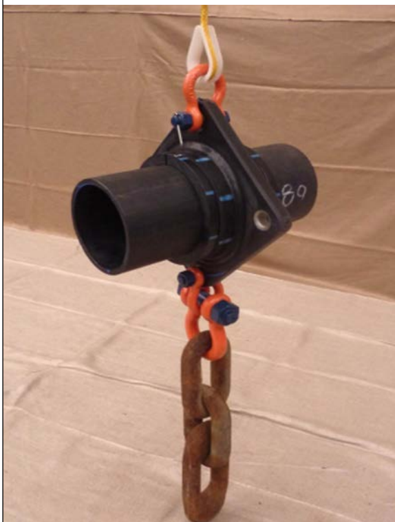
PLATE 37 HDPE connection element for sinker tube. This model shows how the sinker tube (represented by the portion of pipe) is fixed to the sinker rope (in yellow with plastic thimble), and how additional sinkers can be added (such the chain, as shown). The remaining free hole can be used as an attachment point for the net
