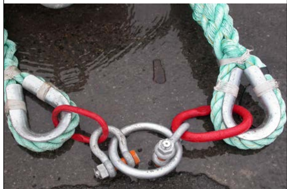
PLATE 18 Steel rings used for connecting eye spliced ropes with thimbles through a pair of shackles. Another shackle then connects the circular ring to the corner plate
