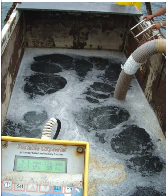
PLATE 101 A large container modified for fish transport. In the foreground, the oxygen meter display can be seen
