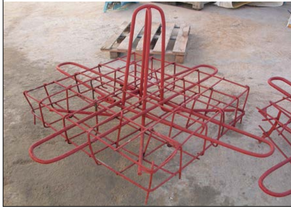
PLATE 4 Iron frame used for industrial concrete block building
