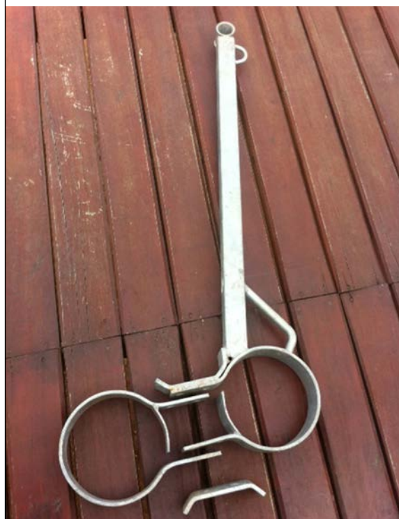
PLATE 28 Disassembled components of a galvanized steel bracket
