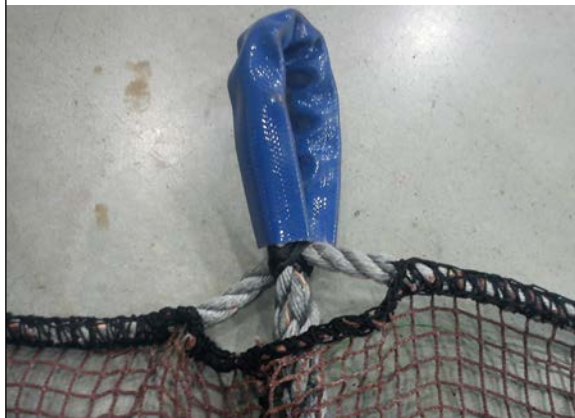
PLATE 62 Top rope loop, spliced with pipe protection
