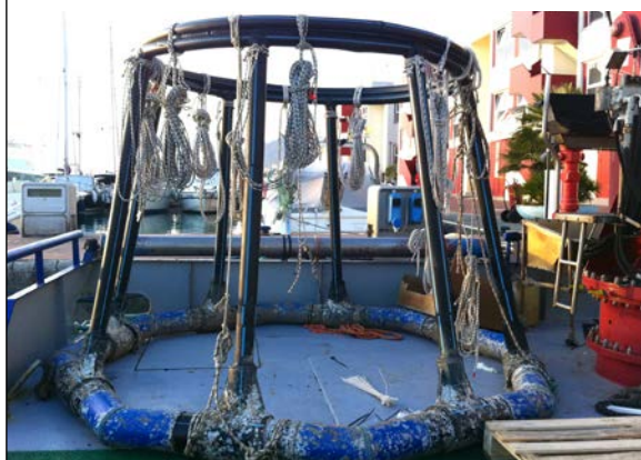
PLATE 80 Bird net floater ready to be installed. Numerous ropes are used to fix it in the centre of the cage
