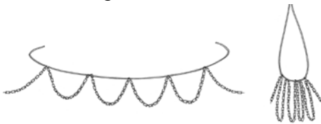
FIGURE 14 Chains can be bunched with a rope passed through every 20–30 links, to permit easy handling with a forklift or crane
