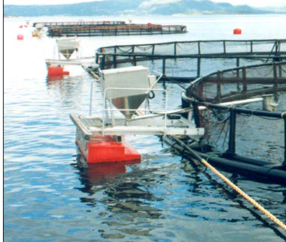
PLATE 113 Feed delivery pipes connecting the centralized feed system with the cages
