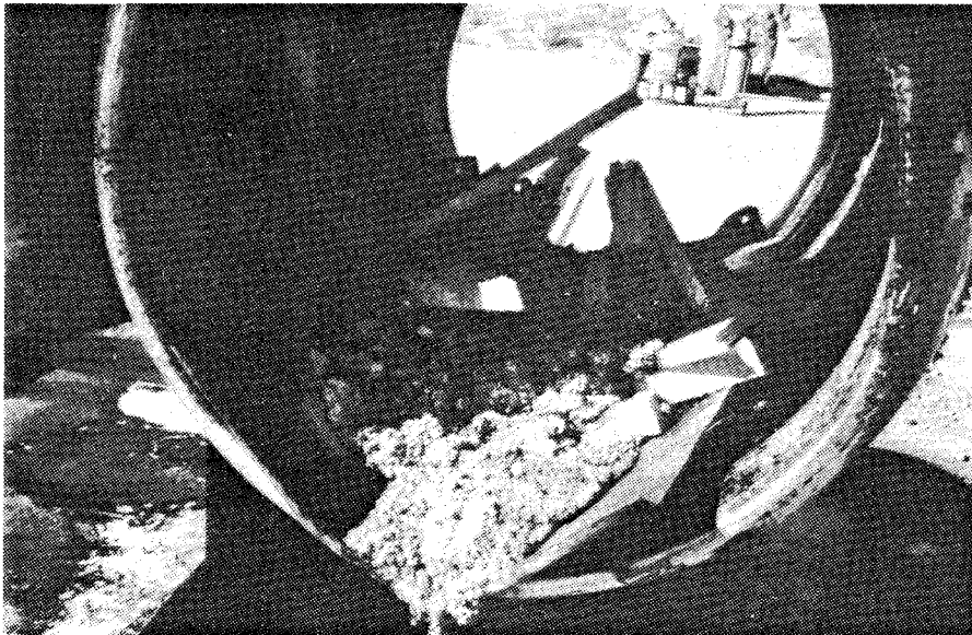
Figure G-6. Residue in Cowling Following Burn.
