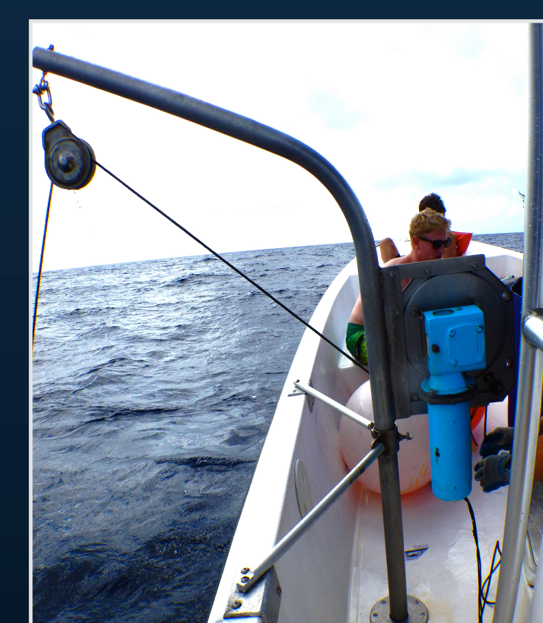
Figure 14: Hauler used for retrieving traps
