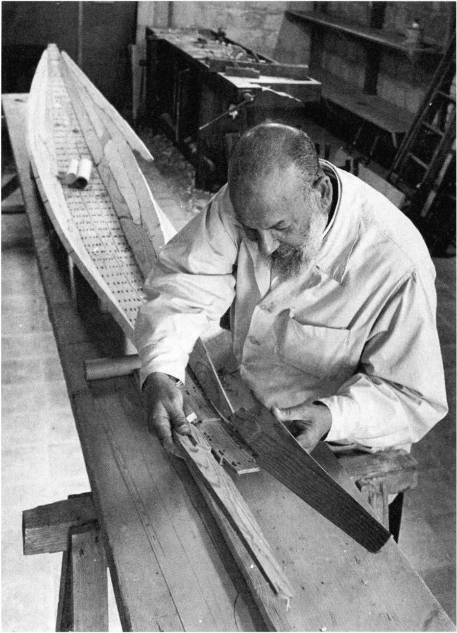
56 Ahmed Youssef Moustafa with a small model of the hull of the Royal Ship. The forward part of the hull is in the foreground and it becomes clear how the curved blades join together to form a prow over which the papyriform sleeve fitted (cf. ill. 78).
