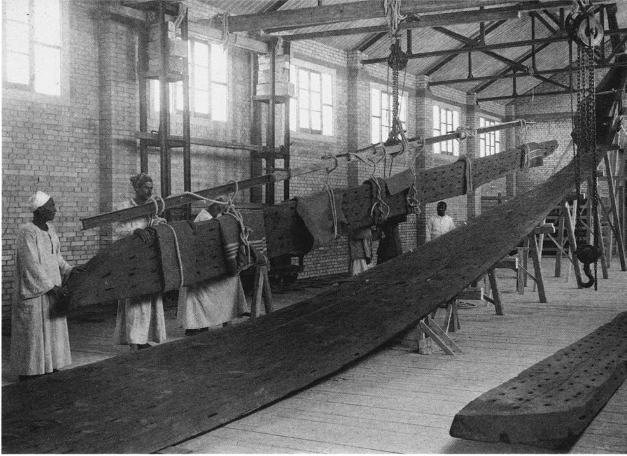
73 The same care was taken at all stages of the reconstruction. During a trial assembly, one of the garboard strakes on the starboard side is moved into place. At each point of contact the ancient wood is protected by blankets and rolls of heavy industrial felt. To avoid undue stress the whole timber is supported by a steel I-beam.
