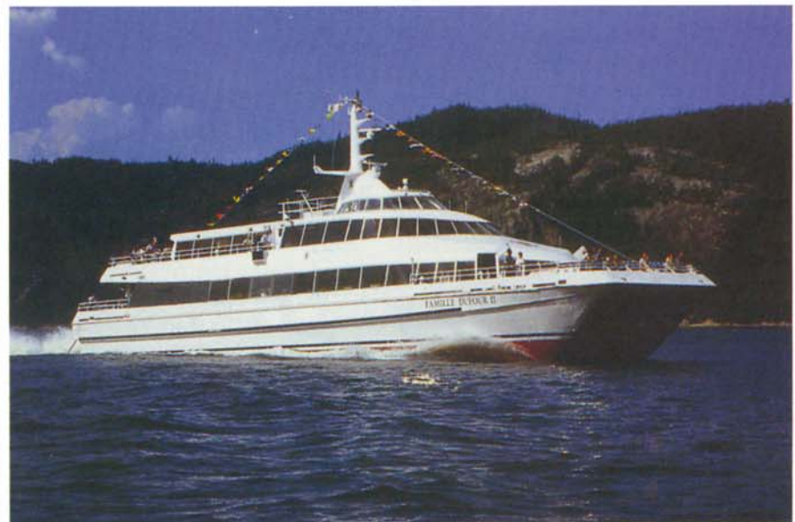
40 metre TWIN HM811 JET POWERED CATAMARAN FERRY "FAMILLE DUFOUR II" TRANSITS THE ST. LAWRENCE RIVER AT 35 KNOTS
