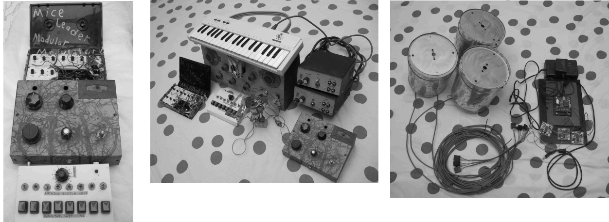
Fig. 2. Control panels closeup, control panel-image generators-midi keyboard interfaces, and optical motion sensors inside buckets with Teleo sensor interface for computer.
