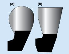
ter elastomeric gasket functions is shown in Figure 5. In the absence of internal pressure, a compression seal is formed as the elastomer is squeezed between the bell and spigot. Under internal pressure, the elastomeric material is redistributed and pushed forward within the pipebell recess. The higher durometer elastomer ensures the seal is firmly seated within the bell recess and that blowouts don't occur; leakage is prevented by compression sealing of the lower durometer elastomer.
