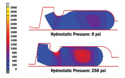
palities also run hydrostatic pressure tests to verify a pipeline's integrity.
