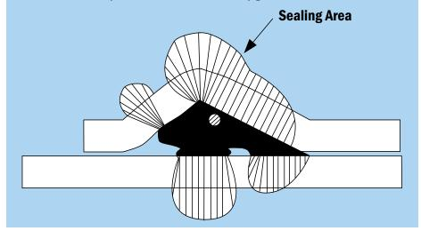
were finally resolved with the introduction of the Rieber-type gasket in the late 1970s. Today, more than 90 percent of PVC pipes in North America use the Rieber joint while less than 10 percent use the dual-durometer type. Rieber is a generic name used to describe a steel-reinforced elastomeric seal that is incorporated in the pipe bell during manufacture, making the gasket an integral part of the pipe.
