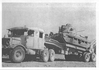
14. A British tank transporter, with a Matilda up, on its way to the workshops. 15. German Pzkw III Special, with long 5-cm gun and spaced armour on the gun mantlet and front superstructure; captured after the Battle of Alam el Halfa.
