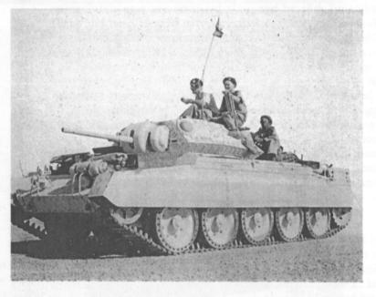
13. British built cruiser Crusader; like Matilda and Valentine, it mounted a 2-pdr gun in a revolving turret.
