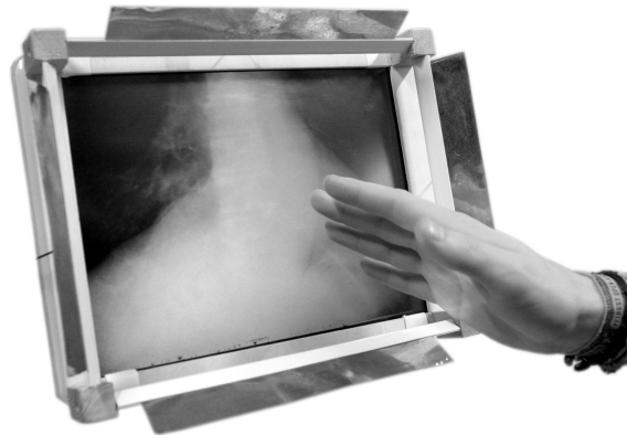
Figure 10. The picture shows a prototype of a screen equipped with capacitive sensing technology. In this example the user navigates (scrolling/zooming) through an X-ray photograph by moving the hand and performing gestures in front of a screen.
