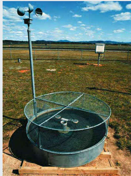
Fig. 4.24. Class A pan at Canberra Airport, Australia. In Australia Class A pans are usually equipped with a bird-guard (as shown). This design is not necessarily used elsewhere and care is needed when comparing pan evaporation measurements from different places (see Ohmura and Wild 2002) (photo: Jeff Wilson)
