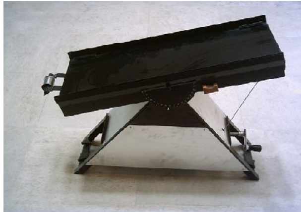
Fig 1. Apparatus for measuring the static coefficient of friction
