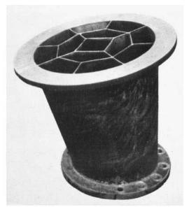
Fig. 11. The Unconventional Bladeless Turbine Nozzle Scroll in the First Model of the Experimental Engine
