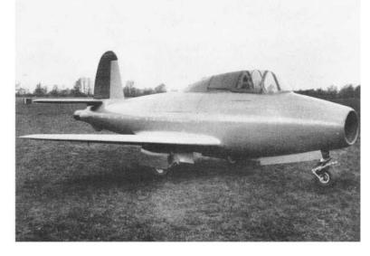
Fig. 41. The Gloster-Whittle Experimental Aeroplane E28/39 (R.A.F. Official, Crown Copyright Reserved)
