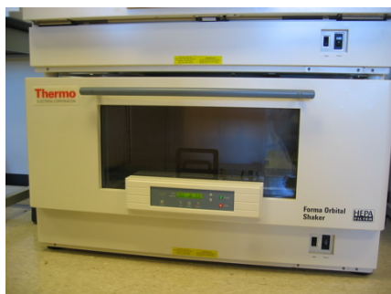
Figure D.5: This Thermo electron shaking incubator is very quiet but only works well at temperatures 35C and above. It is also very slow to start and stop and has an annoyingly long delay between when you push the start/stop button and when it decides “ok I’ll begin stopping now”. We have two stackable ones.
