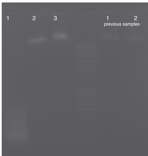
Figure 5.4: Genomic DNA on a 1% agarose gel. The genomic DNA is too long and doesn't run properly. Samples 1 and 2 on the right are from the previous attempt at making genomic DNA. Sample 1 on the left did not have an RNase digestion step (as can be seen by the large amount of RNA)
