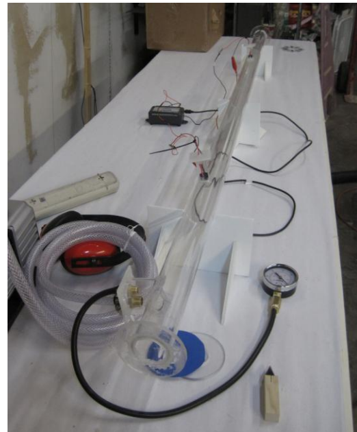
Shock Tube for active drag reduction experiments.
