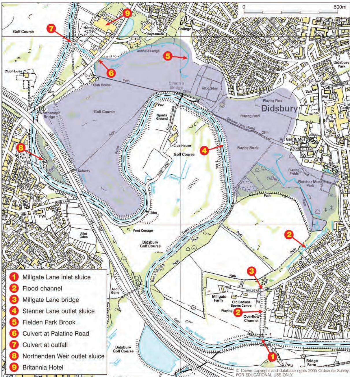
Figure 5: Flood plain map of the River Mersey between Northenden and Didsbury showing the inlet sluice at point 1 and the outlet at point 7.
