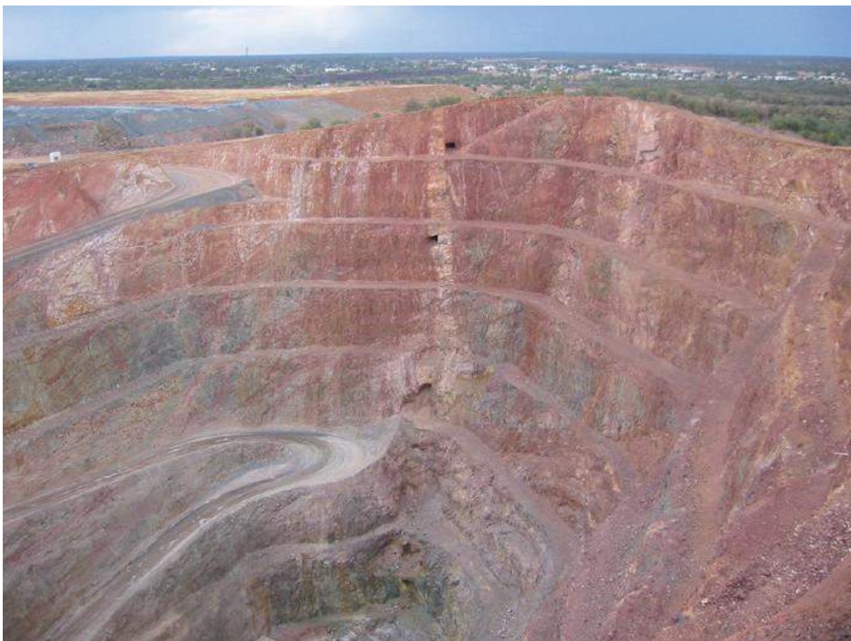
Figure 35: Open pit, New Cobar gold-copper deposit (view NW). This is a Cobar-style deposit hosted by siltstones-sandstones of the Great Cobar Slate. It is structurally controlled and localised in a NNW-trending shear zone with associated ‘pebble’ shears. The top five benches are in oxidised and leached saprolite showing strong ferruginisation, particularly along fractures. The lower section is weakly oxidised saprock. Major quartz vein (near old workings) post-dates the main mineralisation. Photograph by K. McQueen.
