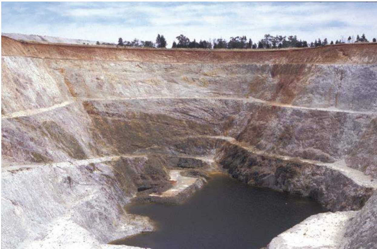
Figure 25: Open pit, McKinnons Tank gold deposit (view to NW). This is a pyritic quartz-vein stockwork system, exploited in the oxidised, supergene gold-enriched zone. Pit walls expose bleached saprolite with minor near surface ferruginisation (iron oxides) and deeper ferruginisation along faults/shears and bedding planes near weathered mineralisation. Primary pyrite is exposed in the lower left part of the pit. The deposit shows primary silicic and sericitic wallrock alteration and weathering-related alteration of sericite (mica) to illite (clay). Photograph by K. McQueen.
