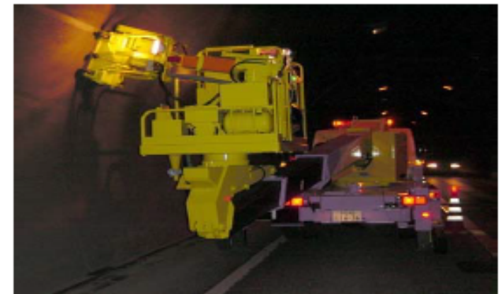
An inspection vehicle carries out non-destructive testing
