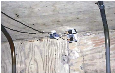
Typical sensor installation in a girder (above); one of the time-synchronized data acquisition modules.
