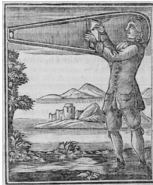
Figure 4: Hooke's portable camera obscura (1694).
