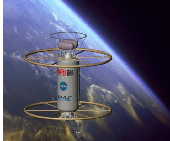
Figure 2 – Artist's concept of the proposed collection system formed of superconducting rings.
