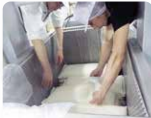
Cloth bags holding fermentation mash are stacked on the fune .
