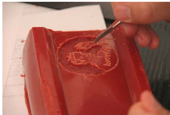
Figure 35: Wax engraving for making Prince Coin , for The Prince of Hampshire (2006).
