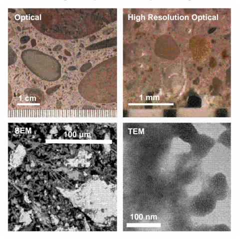
Concrete is heterogeneous on scales from cm to nm
