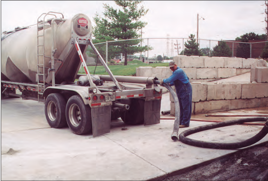
FIGURE 6.5A. Rubber hose used to transfer silica fume from tanker to producer's silo.
