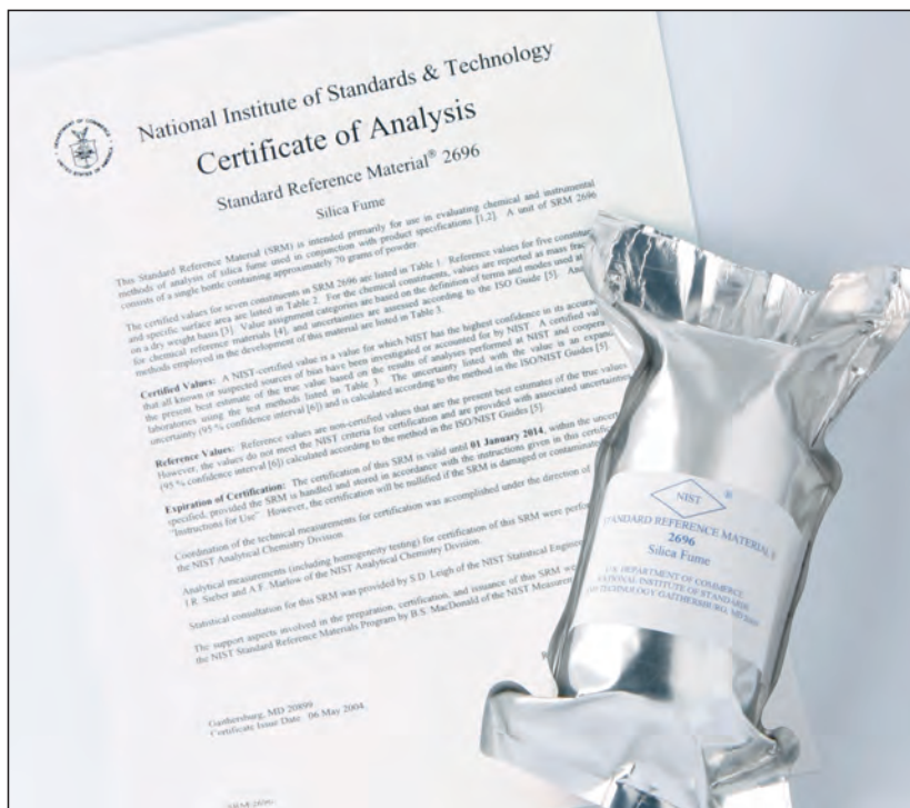
FIGURE 4.5. Silica fume Standard Reference Material (SRM 2696) available from the National Institute for Standards and Technology. Check either the SFA or NIST websites, as listed in the text, for instructions on how to order this material.
