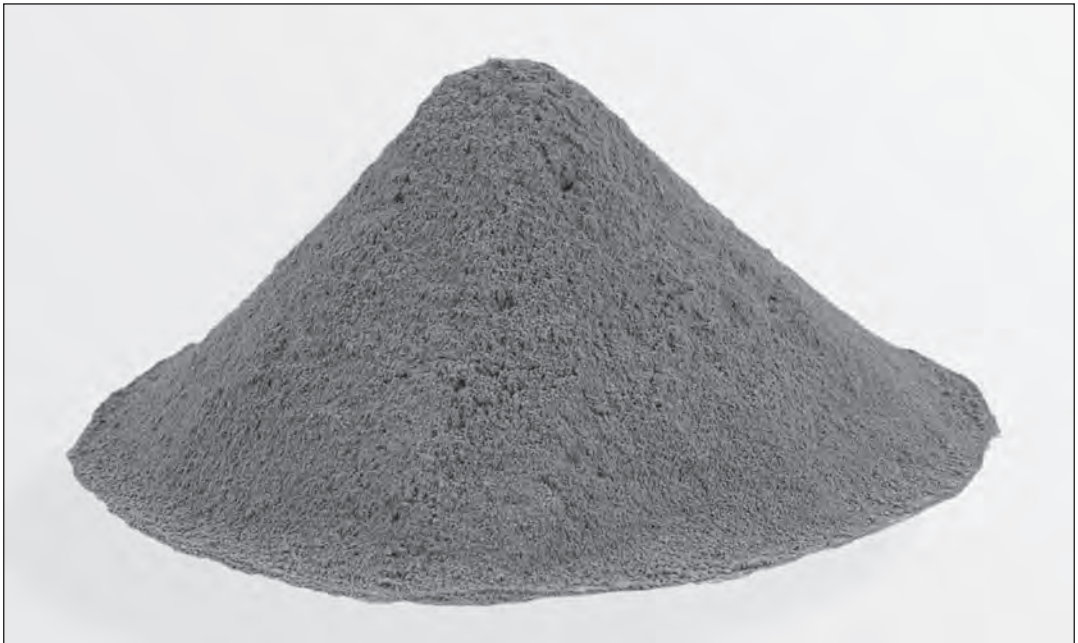
FIGURE 1.1. As-produced silica fume. This is what the material looks like after it is collected.
