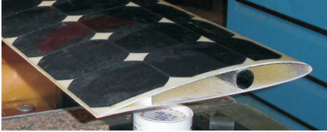
Figure 5.14: Integration of the solar cells during the molding process (AcPropulsion's Solong)
