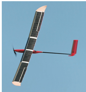
Figure 1.1: The fully functional solar airplane prototype, named Sky-Sailor, developed within the framework of this thesis during an autonomous flight
