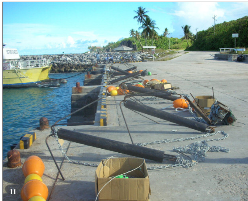
Figure 10: The sub-surface section alongside the surface flotation of the combination sub-surface/surface flotation inshore FAD deployed at Baitisi
