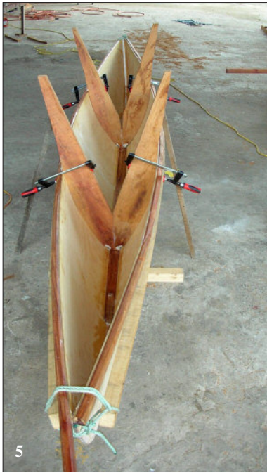
Figure 5: Canoe hull clamped to the construction jig
