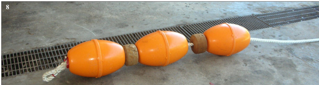
Figure 9: Mooring section for the cheap all-rope FAD before aggregators were connected
